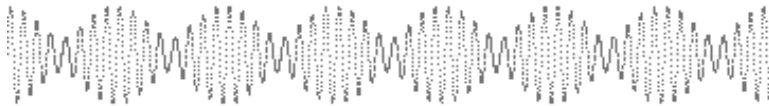
Figure 6.2: This is a plot of \Psi in Eq. (6.6) for t = 0 , which is a “snapshot” of the beat phenomenon. The width of one “packet,” denoted by the horizontal line, is \Delta x as in Eq. (6.7), which can be expressed as 2\pi/\Delta k .
