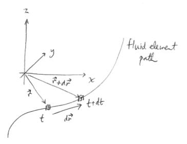
Figure 1: Motion of a fluid element.
