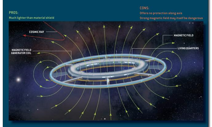
To suppress the field inside the living quarters, the spacecraft designers could add a second, inner electromagnet ring. But the cancellation is only partial and greatly increases the complexity of the system.
