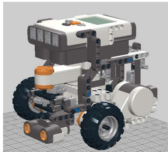
Fig. 1. Design of three wheels robot construction
