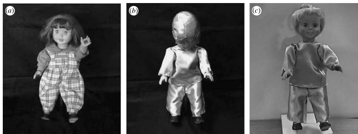
Figure 13. (a) The Robota robot and (b, c) its modified appearances used in the trials with children with autism. The robot's main body contains the electronic boards and the motors that drive the arms, legs and head (Billard 2003). A pilot study showed the use of the robot's sensing abilities and autonomous behaviour was not suitable for our trials, thus the robot has since then been used as a remote-controlled puppet (controlled by the experimenter). A summary of the use of this robot in autism therapy and developmental psychology is provided by Billard et al. (in press). Experiments describing how children with autism react to different robot appearances are reported by Robins et al. (2004b,d).
