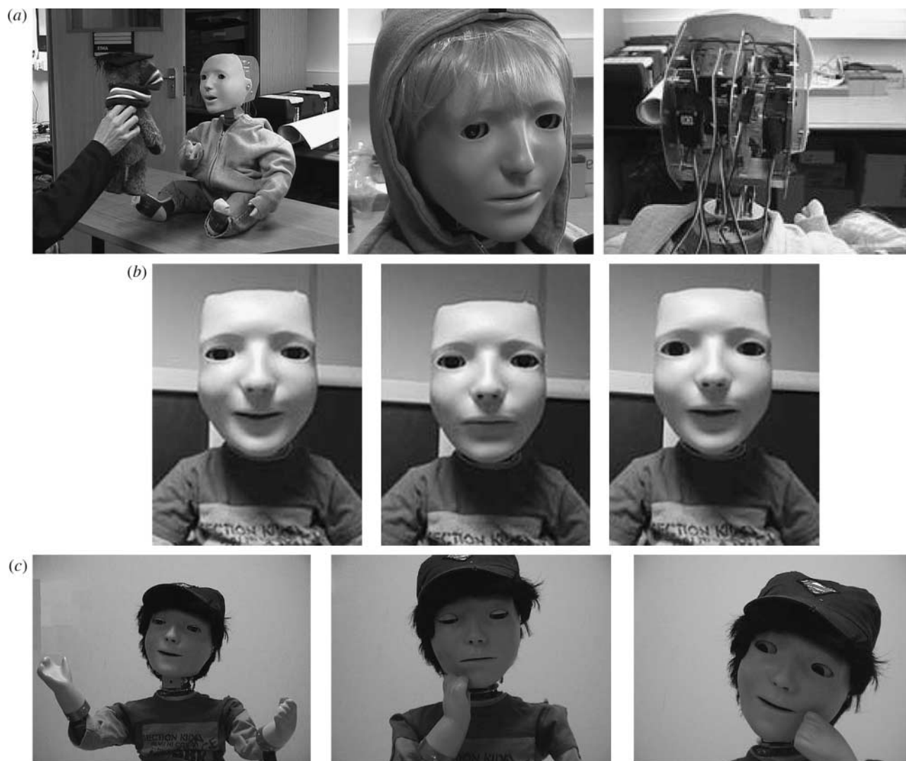
Figure 3. Experimental humanoid robot platform for the study of synchronization, turn-taking and interaction games inspired by child development. Kaspar, a child-sized humanoid robot developed by the Adaptive Systems Research Group at the University of Hertfordshire. (a) Kaspar has a minimally expressive head with eight degrees of freedom in the neck, eyes, eyelids and mouth. The face is a silicon rubber mask, which is supported on an aluminium frame. It has two degrees of freedom in the eyes fitted with video cameras and a mouth capable of opening and smiling. It has six degrees of freedom in the arms and hand and is thus able to show a variety of different expressions. (b) Kaspar's expressions: happy; neutral; and surprised (Blow et al. 2006). (c) Some of Kaspar's expressions using movements in the head and arms.
